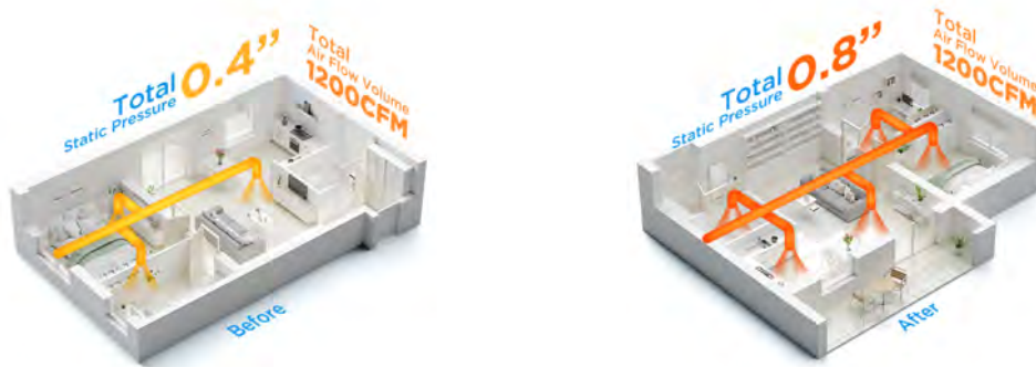
Different Ductwork Designs, Same Air Volume
